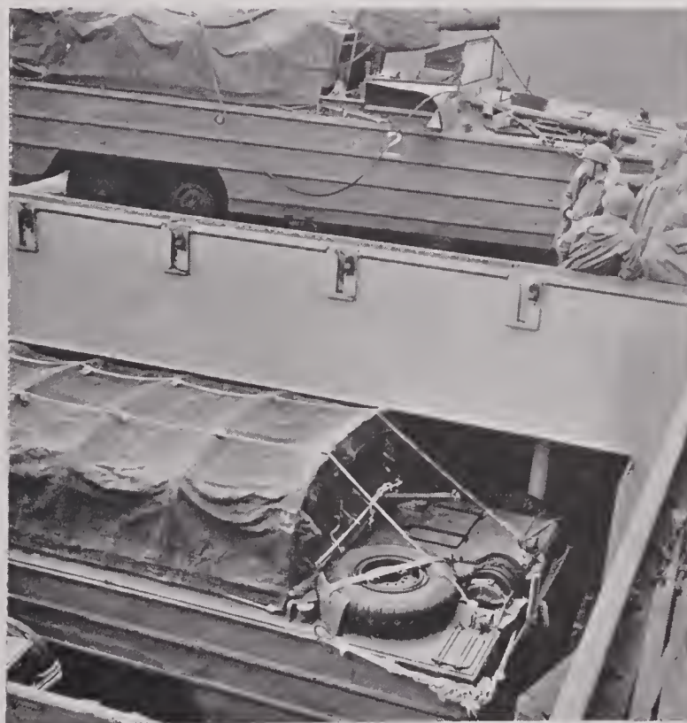
FIGURE 105. Stowage of DUKWs in Liberty ship, in hold and on deck.
